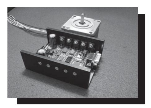
The SMD (small drive) is a bipolar micro stepping drive with Pulse Width Modulation amplifier(PWM) switching at 20 KHz frequency. The drive regulates the current in the motor windings using three different techniques: charging, discharging and circulating. It minimizes ripple current and motor heat caused by the PWM.
