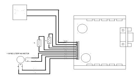
The drive has two connectors on the board; a 10 pin screw tight terminal block for power and the motor. A 9 pin "D" connector for the indexer.
