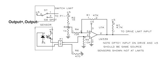
There are 3 outputs available for the user. Output+ connects to the collector of the output photocoupler, while output- connects to the emitter of the photocoupler. See figure 2. The photocoupler has a maximum voltage rating from collector to emitter of 30 volts and has a maximum current of 10 ma.
